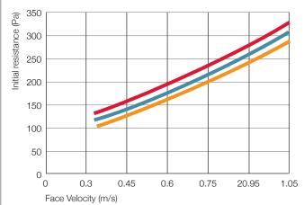
Add 15 Pa to initial resistance for hood construction. Filter depth 125 or 145 mm: 48 mm media pack U16, U15, H14
